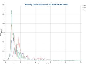
With the VIBRA PC software the measurement data are shown directly in accordance with DIN guidelines. The above graphs show the measured peak values against time, the peak values against frequency (in accordance with FFT method) and the continuous measurement signal (trace) with the accompanying spectrum.
